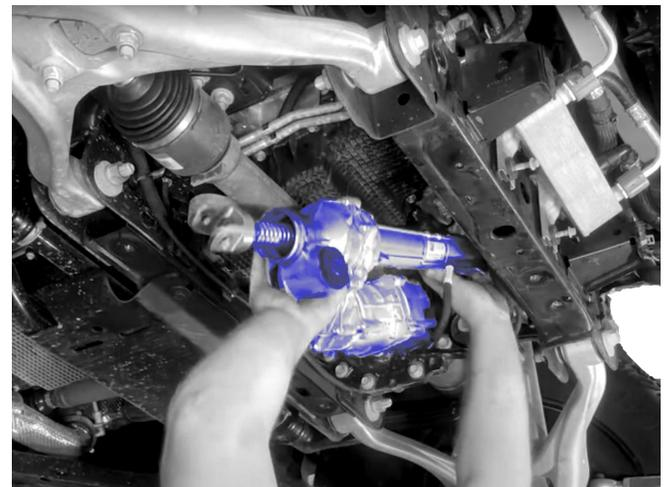
12. Remove rack by pushing it toward the passenger side of the vehicle. Rotate the rack fore and aft as required for the pinion to clear the differential and engine.
