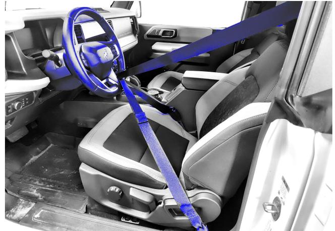
8. Center rack position by straightening the steering wheel. **LOOP THE SEAT BELT THROUGH THE STEERING WHEEL TO PREVENT ROTATION IN FOLLOWING STEPS**
